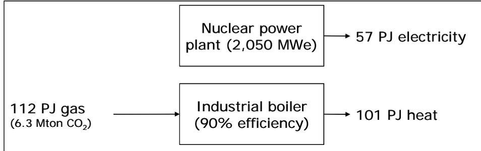
Reference situation with a CHP plant, and the new situation where the electricity is delivered by a nuclear power plant and the heat by a high-efficiency industrial boiler. Assumptions: CHP with an electric efficiency of 27% and a thermal efficiency of 50%. Nuclear power plant (2,050 MWe) running 7,684 hours per year. Industrial boiler efficiency: 90%. CO<sub>2</sub> emissions natural gas: 56.1 kg CO<sub>2</sub>/GJ. CO<sub>2</sub> emissions coal: 97 kg CO<sub>2</sub>/GJ.
