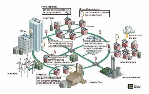
Figure TS-22 | Example of a smart grid, a network of integrated microgrids that can monitor and heal itself. Source: Amin, 2008; see Chapter 15.30
